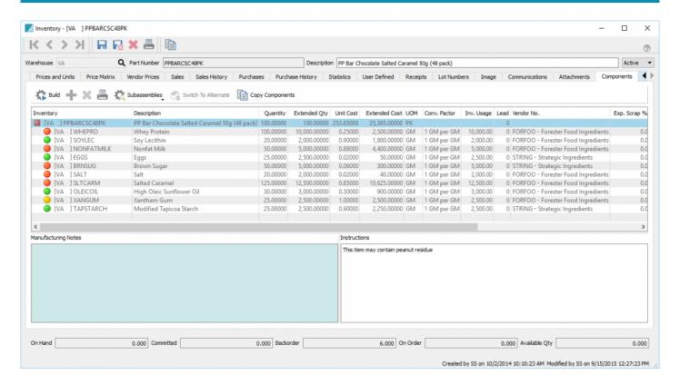
If an item is set as manufactured or kitted it will have a components tab. You can see very visually if you have enough stock to be able to build the item. The green dots mean that there is enough of the component, the red dot means that there is not, and the yellow dot means that there is enough for this build but we are over-committed. There is also an orange dot to indicate that we are short, but a purchase Order has already been issued for the shortage.
