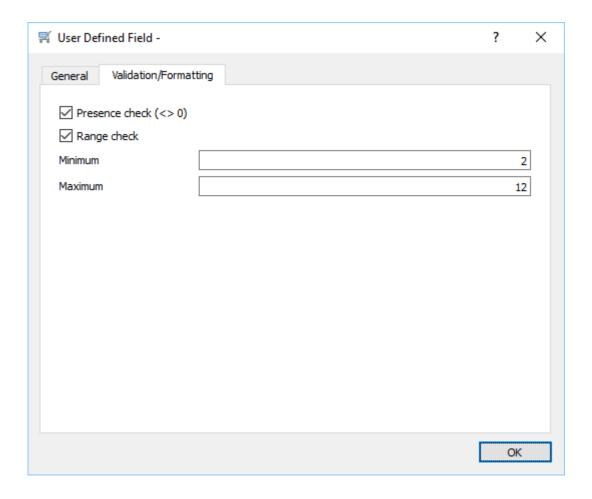
On this field we checked that the field cannot be zero and has to fall between 2 and 12.
