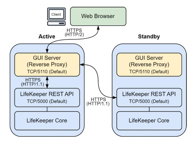
In the LKWMC, the <u>GUI Server</u> and <u>REST API Server</u> components are installed on each node in the LifeKeeper cluster. A user may access the GUI by using a web browser to connect to the appropriate port on any node in the cluster where the GUI server is running. See <u>Connecting to the LKWMC</u> for more details.
