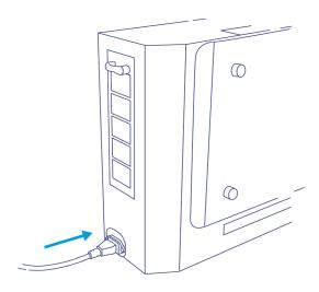
5. Insert power plug into wall socket. Ensure correct mains voltage.
