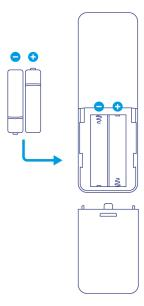
Remove batteries from the remote control if not in use for an extended period.
