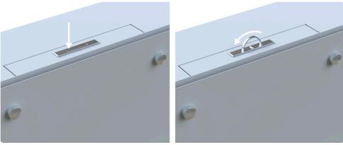
Gently slide the filter tray out of the top of the device.
