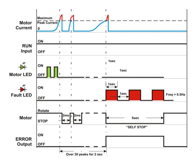
Diagram depicts operation when *CONFIG DIP SW 4* is set to **ON** (Automatic Reset) which causes the motor to automatically restart after forced stop. If *CONFIG DIP SW 4* is set to **OFF** (Manual Reset), then the *RUN* signal must be toggled OFF then ON again to restart the motor.
