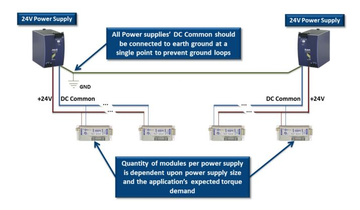
Improper grounding of MDR and/or Power Supply Common may result in premature MDR and/or EZ-QUBE module failure. Proper grounding techniques <u>MUST</u> be observed for all applications
