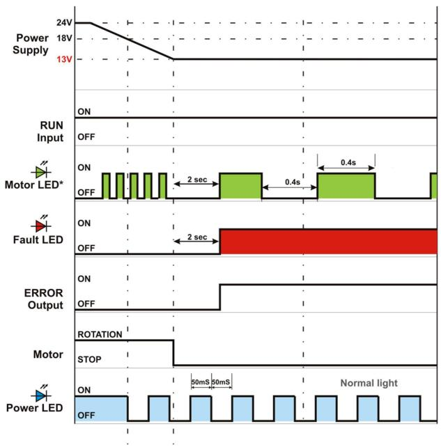
\* Frequency is proportional the rotation speed of the motor
