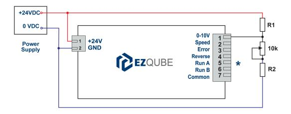
Here are some resistor values to get some common minimum speeds when the potentiometer is set to 0:
