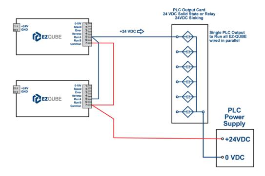
Wiring Multiple Modules with Single Signal for
