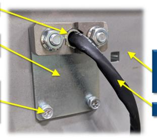
Conveyor frames must be bonded together and connected to earth ground at a single point
