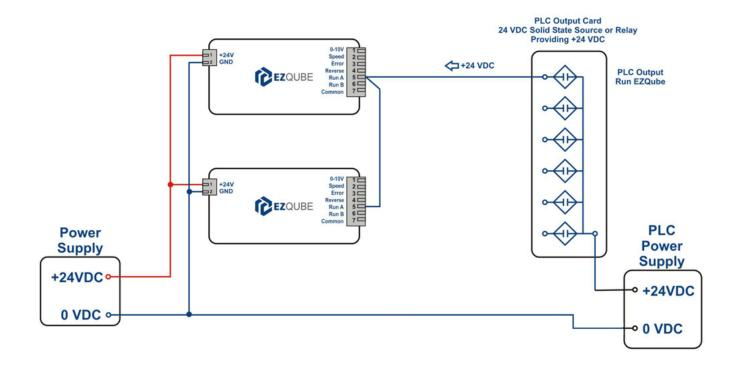
To use the REVERSE input, either RUN A or RUN B must also be energized. Please note that you DO NOT have to de-energize both RUN A and RUN B signals in order to change MDR direction with the REVERSE input.
