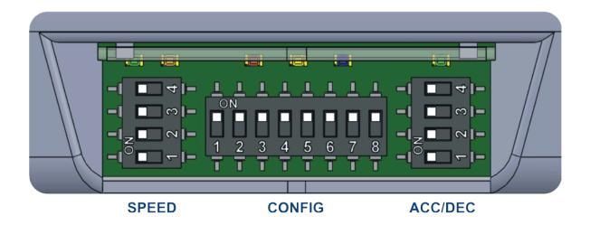
Please note that all switch actions take effect immediately except Switch CONFIG- 2 "Direction of Rotation". It will take effect only when the motor is NOT running.
