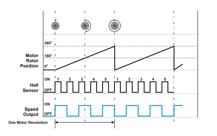
The frequency of this output is shown for both ECO and BOOST modes in the <a href="SPEED DIP Switch">SPEED DIP Switch</a> <a href="Chart">chart</a>
