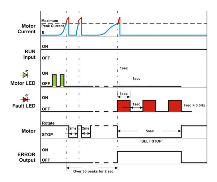
Diagram depicts operation when *CONFIG DIP SW 4* is set to **ON** (Automatic Reset) which causes the motor to automatically restart after forced stop. If *CONFIG DIP SW 4* is set to **OFF** (Manual Reset), then the *RUN* signal must be toggled OFF then ON again to restart the motor.
