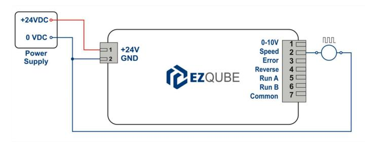
Please note for part number <u>EZ-QUBE-P-MR (Article Number 1510-6020)</u> the Speed output is <u>not a frequency signal</u> but is a <u>maintained digital output signal</u> that is energized whenever the motor is running
