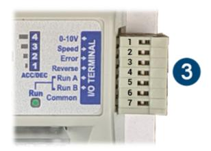
Wire terminals on all removable connectors are "cage-clamp" style requiring a small blade screwdriver to open the clamp to insert the wire
