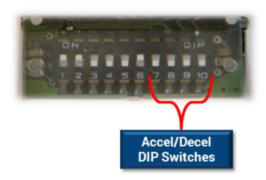
The following chart shows the 16 possible ACC/DEC DIP switch settings for *G* force ramp and the expected ramp time to reach full speed (when accelerating) or to stop (when decelerating) when the motor speed is set to *maximum* (Switch setting item 32 from the <u>Speed DIP Switch chart</u>).
