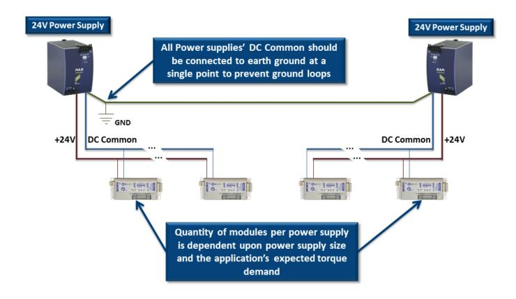
Improper grounding of MDR and/or Power Supply Common may result in premature MDR and/or E-Qube module failure. Proper grounding techniques <u>MUST</u> be observed for all applications
