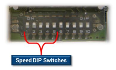
The motor speed is set by the ON or OFF state of DIP switches 1 through 5.
