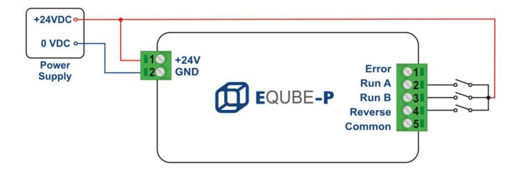
To use the REVERSE input, either RUN A or RUN B must also be energized. Please note that you DO NOT have to de-energize both RUN A and RUN B signals in order to change MDR direction with the REVERSE input.
