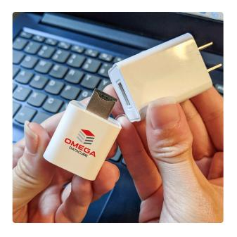
Step 3. Connect your phone's charging cable to both the Omega DataCube USB slot and the phone device.
