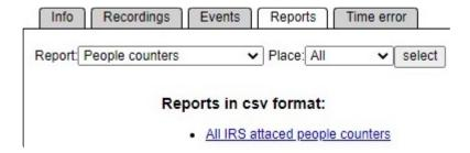
By using the first dropdown menu, a user can select devices such as C3 cameras, people counters, and cameras connected to the Observit IRS.
