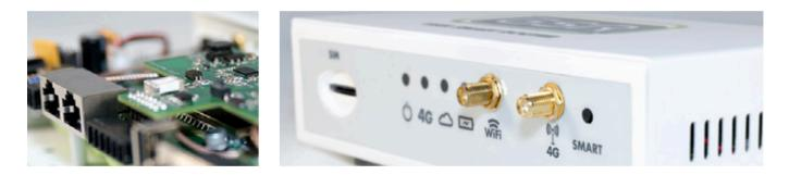
**GSR • GSM Smart Router**® is a device specially designed for elevators and IoT networks. It integrates **2G/3G/4G technology, WiFi** and industrial connectors with the purpose of turning the elevator into an internet device. It is capable of working as a GSM track, an autodialer, can supply connectivity to Advertisim and other compatible devices and is **EN81-28** compliant.
