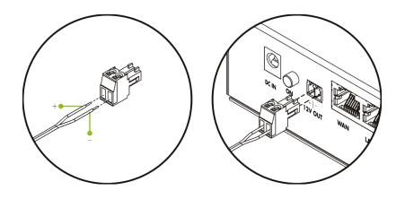
8. Connect the **power supply** to the electric current and DC IN.
