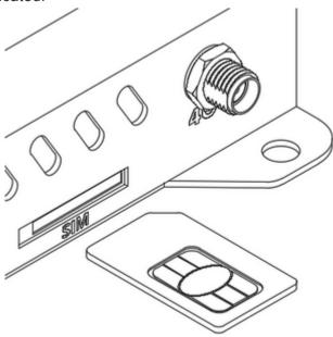
3. Connect the 4G antennas. They must always be connected to the device.
