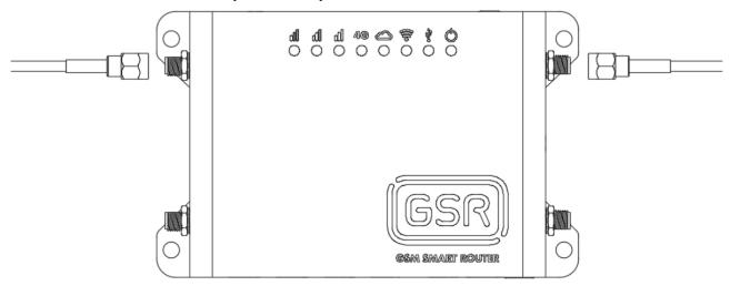
4. Connect the WiFi antennas when connectivity for other devices is needed.
