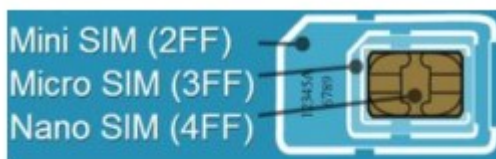
Figure 2: SIM Card Size Formats [Orm09]
