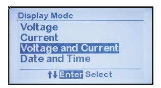
The DISPLAY MODE button is in the same relative location as the METER MODE button on legacy AT10.1 chargers. Its functionality is equivalent in that it determines which measurements are to be shown on the HOME screen.
