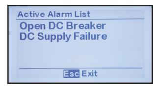
The Active Alarm List can display up to four active alarms at once but it is scrollable to view any additional alarms present.
