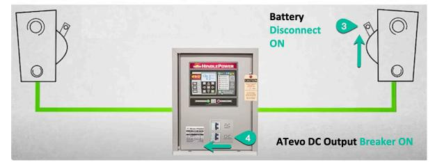
Startup procedure for the ATevo is the reverse of the legacy AT10.1 series chargers.
