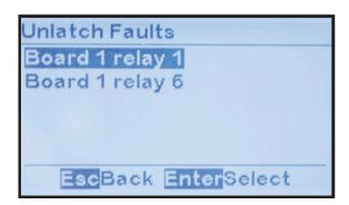
To reset all latched alarm relays: MENU > RELAYS > 'Unlatch all relays (x)', where 'x' represents the number of presently latched relays.
