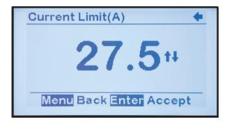
After setting the Current Limit level to the desired value and pressing EDIT/ENTER to save the set point, configuration of Basic ATevo Set Points and Alarms is complete and the display returns to the HOME screen.
