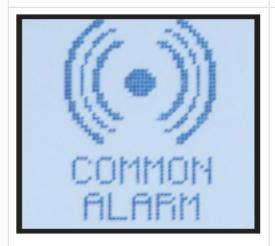
Used to exclude alarms from the Common Alarm activation list. By default, all alarms, when active, will annunciate the Common Alarm. See Section 6.6 for instructions.
