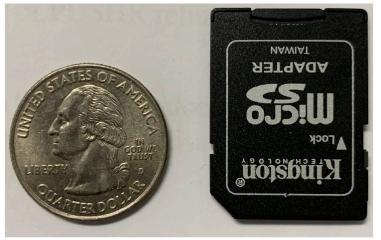
The SDHC card shown above is an adapter for a micro SD card which is also acceptable as long as its capacity is 32GB or less.
