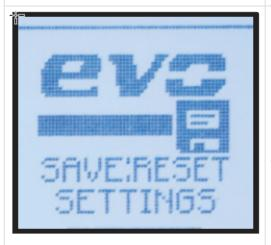
Permits a system backup or restore using an optional SD memory card. All configuration set points, alarm thresholds, and communications settings can be stored on and retrieved from SD memory card. See Section 8.5 for instructions.
