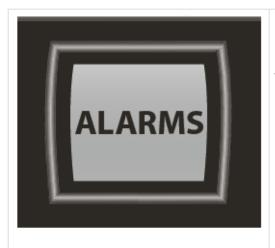
The ALARMS button shows the Active Alarm List – four (4) alarms per page. If more than four alarms are active, use UP and DOWN arrows to scroll through the list.
