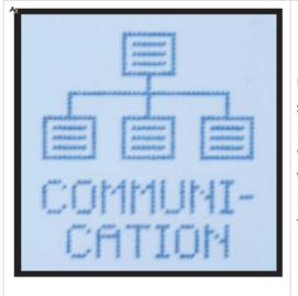
Used to configure optional communications ports. ATevo supports three serial communications ports and one Ethernet port. It shows all communications ports, and whether or not they are assigned and configured. Two (2) of the serial ports support DNP3 and Modbus communications. Refer to the supplementary ATevo Communications Manual for port configuration instructions.
