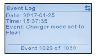
The screenshot above is an example where a left and right arrow icon appear in the top right of the display. This indicates that pressing either LEFT or RIGHT arrow buttons will show additional screens. LEFT and RIGHT arrow buttons are also used when moving between numbers when setting parameters or between characters when setting passwords.
