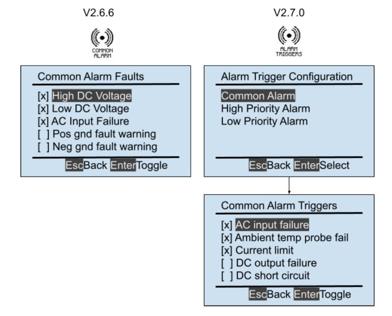
Firmware prior to v2.7.0 navigated directly to common alarm configuration. Firmware v2.7.0 now navigates to a menu that allows a user to select one of the three "aggregate" alarms to configure. The lower right display shown is typical when "Common Alarm" has been selected. "High Priority Alarm" and "Low Priority Alarm" displays are similar. Also new in v2.7.0 is that alarms are listed in alphabetical order. In addition, alarm types that depend on optional hardware are only displayed if
