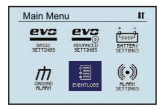
The top-left of the screen indicates the Main Menu is being displayed. The top-right displays an up and/or down arrow icon that indicates that more menu selection icons are available if you continue to navigate in the direction of the arrow(s). In the screenshot above, both up and down arrow icons appear in the top right corner. This indicates that menu icons can be accessed by navigating either up or down from the presently selected icon.
