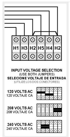
Before you connect ac power to ATevo, inspect the present ac input voltage setting, and confirm the correct jumper positions for the desired ac input supply voltage. The multi-tap ac input voltage setting can be verified without removing the safety shield.
