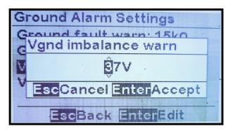
To change the the Ground Imbalance Critical Alarm (measured in Vdc),
