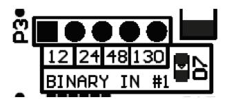
To configure the Binary Input Voltage, move the SHORTING BLOCK to connect the two (2) header pins directly above the voltage rating (12, 24, 48, or 130). Repeat this process for the remaining three (3) Binary Inputs using the associated configuration jumpers for Binary Input #2, #3, and #4.
