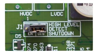
The High Voltage Shutdown jumper (J1) is located center right on the Main Control Board (A1). To change the enable/disable status of the High Level Detect circuit:
