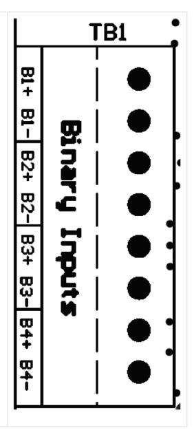
Before wiring the Binary Inputs, verify the Binary Input voltage selection jumpers are configured for the correct input voltage (see Section 12.3.2). Incorrect voltage configuration may damage the Auxiliary I/O Board (A4).
