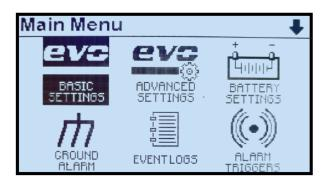
If you are interrupted while adjusting settings and do not press a front panel key for 10 minutes, Edit Mode ends automatically without saving adjustments to any setting not previously saved with the EDIT/ENTER key.
