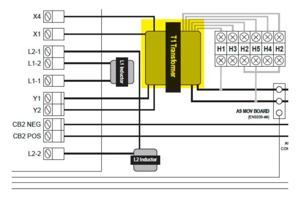
ATevos with the multi-tap ac input option (smart part code 'MT1/2'), feature a terminal block (TB-H#) mounted above the AC Input Circuit Breaker (CB1) for voltage selection. Jumper positions are shown on silkscreen to right of Power Isolation Transformer (T1). See Section entitled ATevo with Selectable Input Voltage for details.
