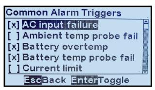
If an '[X]' appears to the left of the alarm, it will activate the COMMON ALARM. If '[]' appears, it will not activate the COMMON ALARM.
