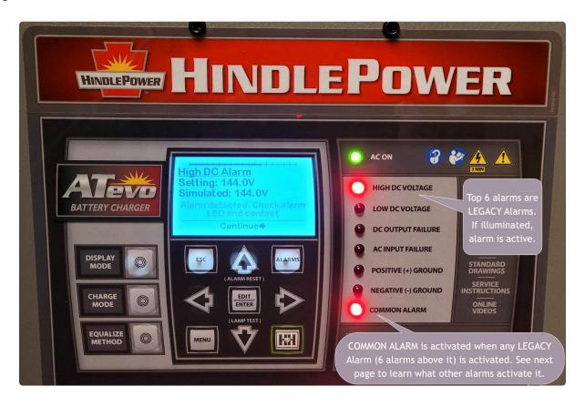
The GREEN AC ON LED indicator, and the six (6) RED Legacy Alarm LED indicators are summarized in the table in Section 7.3.
