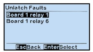
To reset all latched alarm relays: MENU > RELAYS > 'Unlatch all relays (x)', where 'x' represents the number of presently latched relays.
