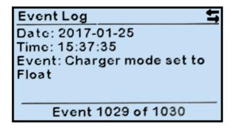
The screenshot above is an example where a left and right arrow icon appear in the top right of the display. This indicates that pressing either LEFT or RIGHT arrow buttons will show additional screens. LEFT and RIGHT arrow buttons are also used when moving between numbers when setting parameters or between characters when setting passwords.
