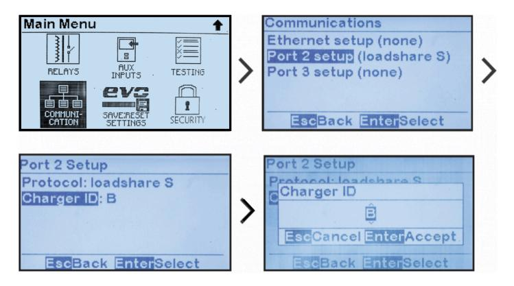
Press the EDIT/ENTER button to accept the new selection. Press the ESC button to return to the previous screen. If a port setting was changes, the ATevo will prompt to RESET. Select YES to RESET the ATevo. The new port settings will not become active until after the ATevo is RESET.
