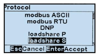
Press the EDIT/ENTER button to accept the new selection. The charger ID may now be changed. Press the ESC button to return to the previous screen. If a port setting was changed, the ATevo will prompt to RESET. Select YES to RESET the ATevo. The new port settings will not become active until after the ATevo is RESET.
