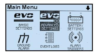
The top of the screen indicates the Main Menu is being displayed and to the far right of 'Main Menu' an up and/or down arrow icon is displayed. The arrow icon(s) indicate that more menu selection icons are available if you continue to navigate in the direction of the arrow.
