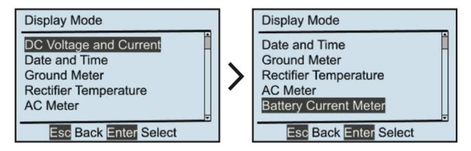
The DISPLAY MODE button is in the same relative location as the METER MODE button on legacy AT10.1 chargers. Its functionality is equivalent in that it determines which measurements are to be shown on the HOME screen.
