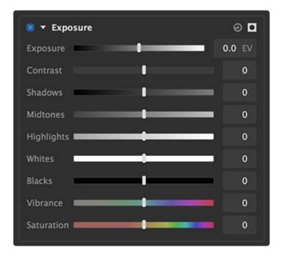
• **Exposure**: This either brightens or darkens the entire image. It does so in such a way where every stop (EV) is a doubling (when increasing) or halving (when decreasing) of the brightness. This better matches the behaviour of exposure in cameras.
