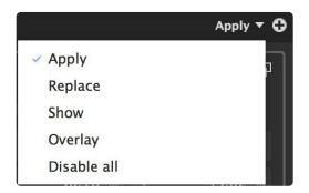
The display mode menu at the top of the masks section controls how the masks are displayed on the canvas. The menu shows the currently selected option, which by default is Apply. Thus the appearance of the menu will change if you have a different option selected, but its location remains constant.
