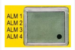
Q-tag Quad is shipped in its so-called "Sleep Mode". This will be observed by the constantly flashing dot (running indicator) on the display.
