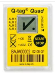
The active recording is shown by the  $\checkmark$  (OK symbol) and the flashing dot on the display.
