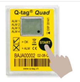
The device is activated by pressing the START- button for at least 2 seconds.
