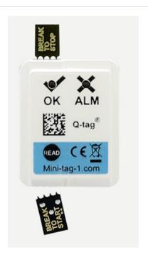
The device is started by the START break-off tab (the tab is labelled BREAK TO START) being completely broken off.
