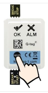
The device is stopped by pressing the READ button (with the edge of a fingernail) for 6 or 10 seconds (standard).
