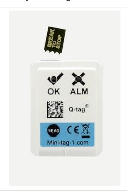
The device is stopped by the STOP break-off tab (the tab is labelled BREAK TO STOP) being completely broken off.
