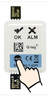
The device is started by pressing the READ button (with the edge of a fingernail) for at least 3 seconds.
